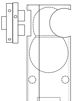
Use a hollowing tool to cut the inside of the drilled hole to fit the 60mm diameter shape of the head you will make later. Sand this inside surface. Remove the wood from the chuck.
