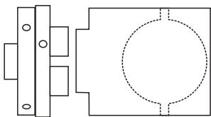
For the head mount the 80 x 80 x 100mm piece of wood in a chuck. Turn it to be round and close to 80mm diameter.
