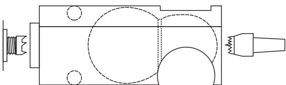
Mark the centres on both ends of the wood and mount it between centres. Turn the wood to a bit more than 80mm diameter. Mark pencil lines around the wood at 10, 40, 60, 100, 130, 140, 163 and 195 mm from the headstock end. Create a 10mm long x 46mm diameter spigot on the headstock end.
