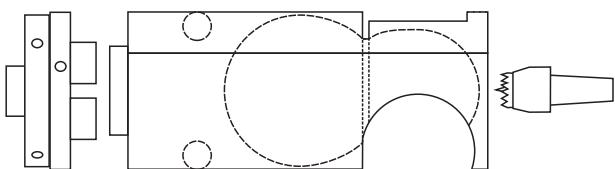
Mount the wood in a chuck. Keep the tailstock up for extra support. Centrally between the 130 and 140mm lines use a parting tool to cut down to create a 55mm diameter for the neck of the cat.
