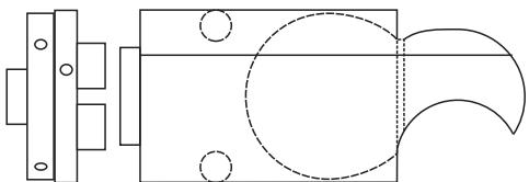
Trim off the tailstock end at the 195mm mark. At the 163mm line turn the wood to be 65mm diameter. Make the head end to be spherical and about 65mm diameter.
