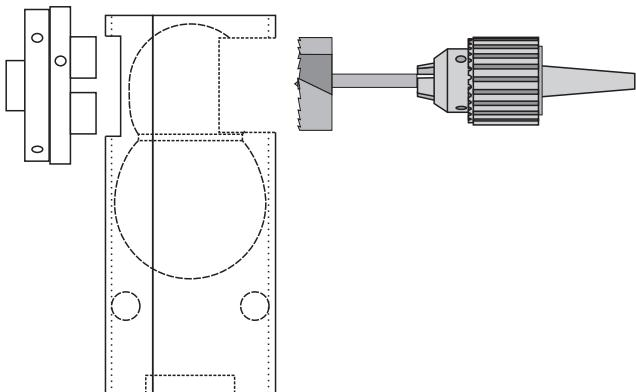
Mount the wood on a 50mm chuck expanded into the 53mm Forstner bit hole. Now drill a 50mm diameter hole 30mm into the wood.
