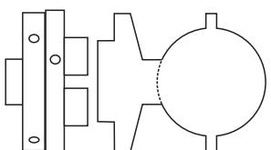
Turn the head to be a 60mm diameter sphere, but with a 4mm thick flange extending about 10mm from the centre of the sphere. Sand these surfaces. Part it off and hand sand the parting cut.
