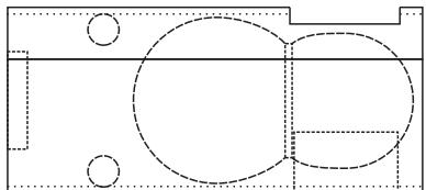
Use a 53mm Forstner bit to drill a 10mm deep hole centred 163mm from the headstock end on the thinner side of the paper joint.
