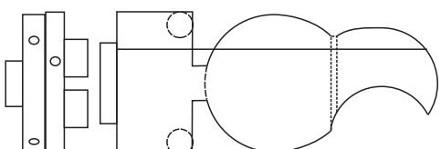
At the 100mm pencil line turn the diameter to be 80mm. Make a curving cut from there to the parting tool cut at the neck of the cat. Make a further curving cut from the 100mm line nearly to the tail of the cat to make the body an 80mm sphere. Sand all this area. Part the work off but keep the wood in the chuck to make the tail of the cat.
