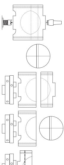
Mount the wood between centres, turn it to round with a spigot on both ends. Insetting the spigot on the headstock end can make later handling of the jig easier. On the tailstock end of the wood draw the diameter of the sphere you intend to make. Draw another line half way between that diameter line and the outer edge of the wood. Now use the index on the lathe to mark this line into quarters. At those points drill four holes the size of the bolts you have, from end to end of the wood.
