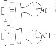
**Make the head oval**. Put the holes for the ears uppermost. Bring up the tailstock to almost touch the wood. Ease the grip of the chuck and raise the tailstock end of the wood by 5mm. Tighten the chuck. Turn 5mm of wood off the upper side of the head. Repeat for the lower side. Sand all surfaces. Decorate the head with eyes, mouth and colours of your choice.
