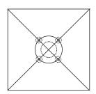
**SHOULDERS.** Mark and drill the two shoulder pieces as follows. Mark the centre on the proposed inside of the shoulders with diagonal lines from the corners. From the centre draw a circle with a 20mm radius to get a 40mm diameter circle. At each point where the circle crosses the diagonal lines drill an 8mm hole to a depth of 10mm. From the bottom of each of those holes drill a 3.5mm through the wood. At the centre of the circle drill a 26mm diameter hole to a depth of 15mm.
