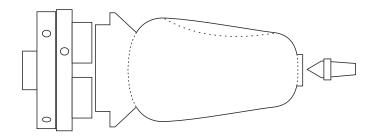
Mount the block in a chuck and turn it to the shape of the underside of the duck body. But leave a 25mm wide uncut area at the narrow end.
