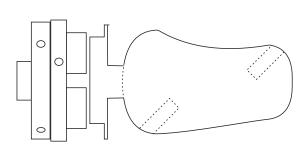
Return the wood to a central alignment. Finish the narrow end and begin the parting cut for the wider end. Sand and finish all this area. You can drill the leg and neck holes now, or do this later. A Brad Point drill is recommended. The holes are at about 45° to the alignment of the wood. Part it off and hand finish the parted area.
