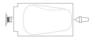
**Body:** Start with a block that is 110 long and 60mm square. Mount it between centres, turn it round and turn an 8mm long spigot on one end.
