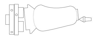
Check the grain showing in the wood to see which area will look best as the duck's chest or bum. Move the wood 10mm off-centre at the narrow end in the direction needed to keep the good grain area. Turn a shallow curve that will be the back of the duck.
