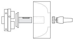
Put a short pin chuck in a four-jaw chuck fit it into the drilled hole in the stone. Bring up the tailstock against a scrap of wood to further secure the stone.
