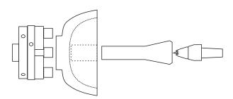
Use wooden or plastic jaws in a chuck to hold the foot of the bowl. Make a wooden dowel addition to the tailstock and bring that up into the drilled hole to better hold the block on the lathe. Hollow the block but keep the wall thickness at 20mm or more. Remove the tailstock only for the last few cuts and to sand the inside.
