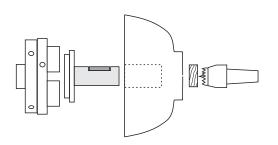
Turn the outside to shape. Sand. Remove the stone from the lathe.
