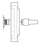
Mount a 70 x 70 x 15 mm piece of dark wood between centres and cut a spigot for a 50mm chuck on one side
