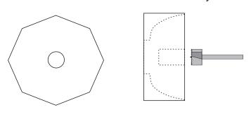
Start with a block of stone 130 square and 60mm thick. You may saw off the corners for easier turning. Drill a flat-bottomed hole from the face side to about 25mm from the planned outside edge of the bottom of the bowl.
