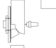
Attach the wood to a faceplate. Hotmelt glue is recommended. Or secure a strap over the square end of the block. To ensure that the centre of the bowl is at the centre of the faceplate bring the tailstock up to the central mark you made. Add glued-in support blocks around the bowl.
