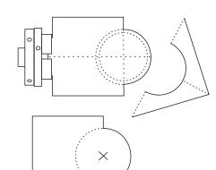
Remount in a chuck and cut the emerging part to an exact hemisphere. Use a template to ensure a perfect hemisphere and the correct dimensions. See "Circle Template" on https://sawg.org.nz/tipsnjigs/ Sand this surface.
