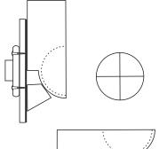
Hollow the bowl. Make yourself a template to ensure an exact internal hemisphere and correct wall thickness. Sand and finish the inside.
