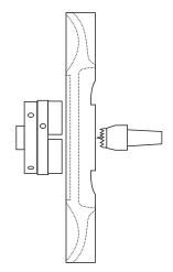
Start with a wood thickness of 35mm. This allows for a 15mm dish in the biscuit tray and space under the edge for easy pickup of the board.
