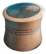
Hollow out the base 40mm diameter and 40mm deep. Turn the rebate for the lid 48mm dia x 6mm deep. Sand and finish inside the base. Set this part aside. Mount the lid held by the spigot on the contrast colour insert. Turn the inside to fit the base. Sand and finish the inside. Keep this part on the chuck.
