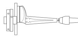
Slide the jam chuck and box top off centre in the chuck jaws. Rotate the box top and slide the jam chuck to bring the offset mark for the finial perfectly on centre. Bring up the tailstock to hold the wood in position. Tape the box lid to the jam chuck. Cut the bulk of the wood away on the top of the box. Keep the lathe speed up to make this hit-and-miss cutting easier.
