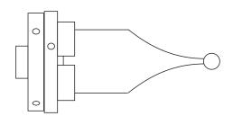
Turn a sphere of about 20mm diameter on the end of the wood. Slope the supporting wood well back to give clearance for drilling holes in the sphere. Turn this support wood as thin as possible bearing in mind the drilling to be done. Sand the sphere. Paint it white and sprinkle on a layer of glitter while the paint is wet.
