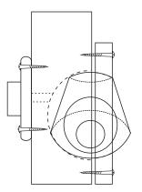
For each of the remaining three holes repeat this process. Align each one with the dowel then drill and then cut. Sand and finish each one as you progress.
