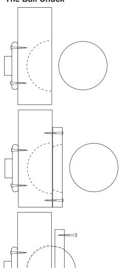
Make a circular template to exactly 100mm diameter. Use a single piece of wood, or mdf and scrap wood, to make a block at least 70mm thick and 200mm square. Mount this on a faceplate with that faceplate 22mm offcentre and exactly on the centre line drawn on the wood. Cut a curve into this wood so that half of the diameter of the template is in the wood but it is not a tight fit. You should also have 20mm thickness left between the bottom of this curve and the faceplate.
