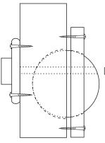
Put the ball into the chuck and align one of the 10mm holes with the 10mm hole in the chuck by passing a 10mm dowel through both. You may check this alignment by bringing the tailstock up to the centre of the dowel end.
