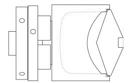
Jam fit the spinning top into the body of the box. Note that the edges of the top are proud of the box sides so that the surface of the top may be finished and sanded.
