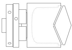
Use a fine parting tool to part the spinning top from the body of the box.
