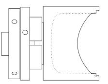
Set the parted off spinning top aside and hollow a little of the box body and then prepare it for use as a jam chuck to take the spinning top.
