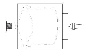
Start with a block of wood about 80mm square and 90mm long. It is best to have the grain along the longer axis but will be ok with crossgrain.
