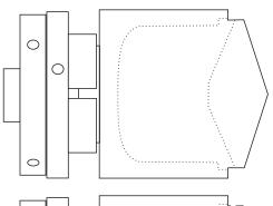
Shape the outer end of the wood to be the underside of the spinning top. Cut a little down the sides too. Note that this spinning top will be jam chucked into the box later so judge the diameter of it for that fit. Sand, decorate if desired and finish the underside and edges of the planned spinning top.
