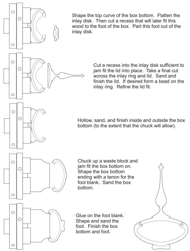
If desired, jam fit the lid into a waste block to finish the underside. Or sand this area by hand.
