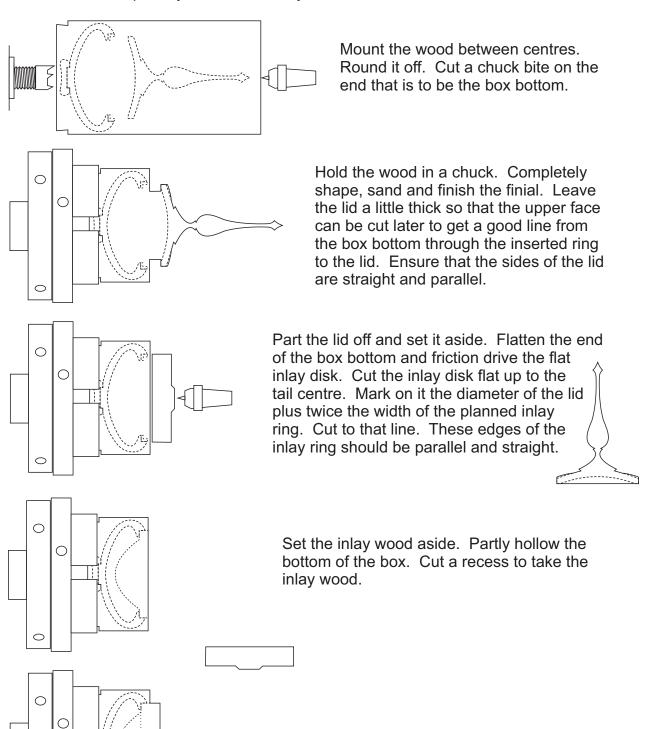
Fit and then glue the inlay disk into the box bottom.
