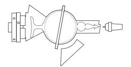
Turn the finial area down to round. Continue to use the section of Circle Template to ensure the curve of the box is correct.
