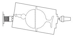
Remount the block between centres with the wood on the diagonal set. Cut a second chuck bite on the bottom. Keep the first chuck bite in good order. To get two chuck bites on the foot end both need to be short. Ensure they are both exactly the correct diameter for the chuck you plan to use. Keep the tailstock up as much as possible throughout this project.
