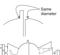
Note, for a spherical finished box, the diameter of each hemisphere where it meets the Saturn Ring must be the same. You need to allow for the thickness of the wood taken out to cut the box to two halves, and the wood needed to fit the lid into the bottom, before the curve of the top part can begin.
