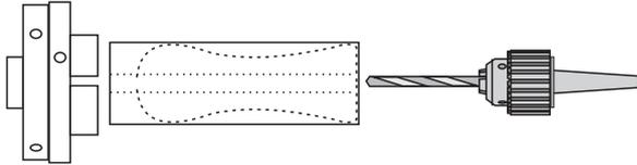
Start with a piece of wood about 40mm square and 120mm long. Grip this in a chuck. Drill a 7mm hole down the entire length (larger if you plan to use thick wool).
