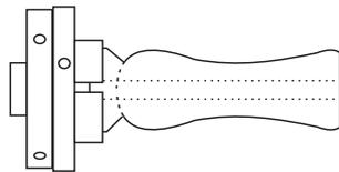
Cut the end nice and smooth. Turn the length of the wood to a nice hand-holding shape. Sand and finish the turned area. Be sure to sand into the drilled hole.
