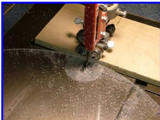
Using a plywood stop that I clamped to the table of my band saw, I proceeded to cut all the slots into the edge of my index wheel. For the first series of cuts the stop was ¼" from the back of the blade. For the remaining set of slots, the stop was positioned right at the back of the blade so that there was a significant, visible difference in size between the slots.
