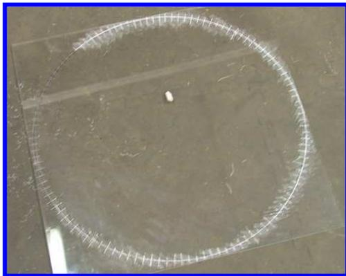
I marked the 120 segments with a scratch awl and then marked the 240 segments with a "Sharpie" felt tip pen. To enhance the circle and the segment lines prior to cutting, I used white chalk which I rubbed into the scratches on the surface of the Plexiglas.
