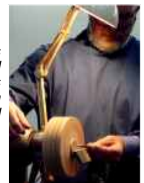
Jim Manley demonstrates his method of creating the ideal curve on a bowl using a series of vertical divisions drawn on the side of a prepared bowl blank.
