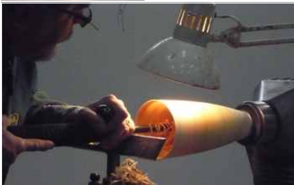
Rolly shows his mini-hollower at work on a thin-walled vase, with the aid of the strong light (Below)
