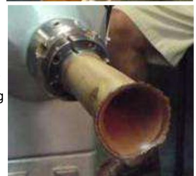
The hollowing and sanding completed, inside and out. Dick uses a combination of long, powered sanding rods and attachments for the inside.
