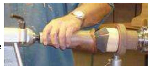
The tail stock is brought up to secure Dick's home-made cup shaped chuck to fit the mouth of the reversed vase and with a protective rubber shield.
