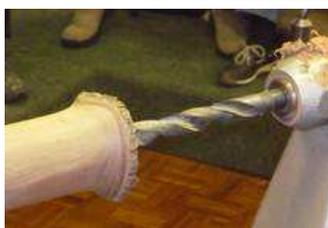
Drill out the centre to the required depth to facilitate hollowing. This drill has a #2 Morse taper to fit the tailstock.
