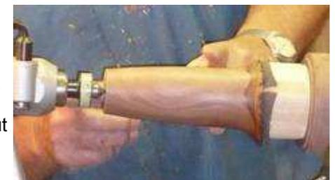
The base can now be finished (at low speeds), parted off with a slight undercut and have a finish applied.
