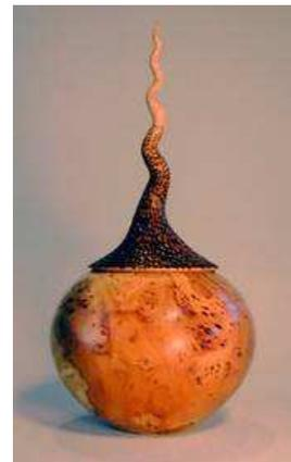
Turn a solid ball with a spigot on the end - *photos 1,2*. Reverse the spigot into a scroll chuck and hollow from other end - wall 10mm thick, using tools of choice. Bevel the edge of the opening so the inner diameter of the opening matches your chuck's minimum grip in expansion mode and the outer rim is about an extra 13mm diam. - *photo 3*. Finish inside and out, working through the grits to 600 on the exterior - *photo 4*. Remove from the chuck and set aside.
