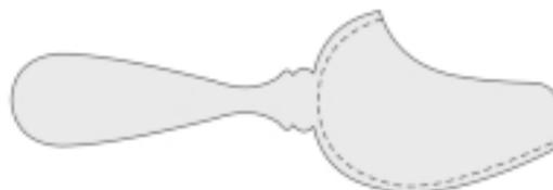
Bandsaw off the unwanted part of the scoop. Sand the cut edge to shape and add your desired finish.
