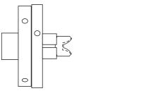
Mount the parted-off top in a small chuck and hollow the inside. Take care to preserve, untouched, the outer 2mm of the parting cut. If you have a morse taper to mount this chuck in the tailstock, keep the wood in the chuck and mount it in the tailstock.
