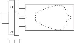
The overall size of the bud vase is your choice. Start with a block that is about two times longer than its diameter and has the grain running lengthwise. Mount this in a chuck. Bring up the tailstock if you need additional stability.
