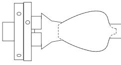
Cut the basic shape except the top. If the foot is to be narrow then it may pay to leave some thickness there too. It is important to visualise and cut the correct curves at this stage.
