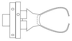
Hollow the inside. Take care to preserve, untouched, the outer 2mm of the parting cut. Thin walls will result in a very light final product. Leaving some weight in the bottom can assist the final balance. Keep the work in this chuck and remove the chuck from the lathe.
