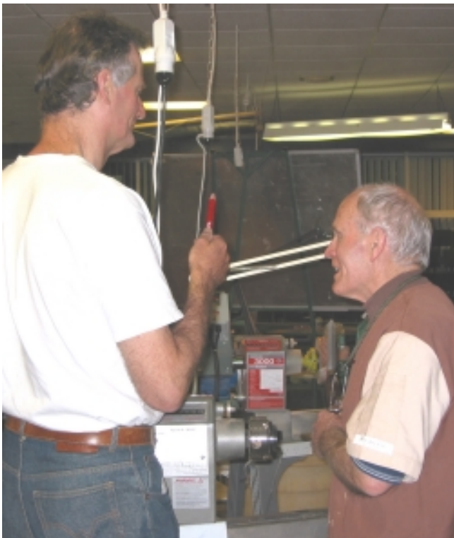
Both these turners would benefit from changing the height of this lathe.
