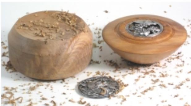
And the tea light. A metal insert is highly desirable for all candles. Lines in the top with a skew tip quickly added to the looks.
