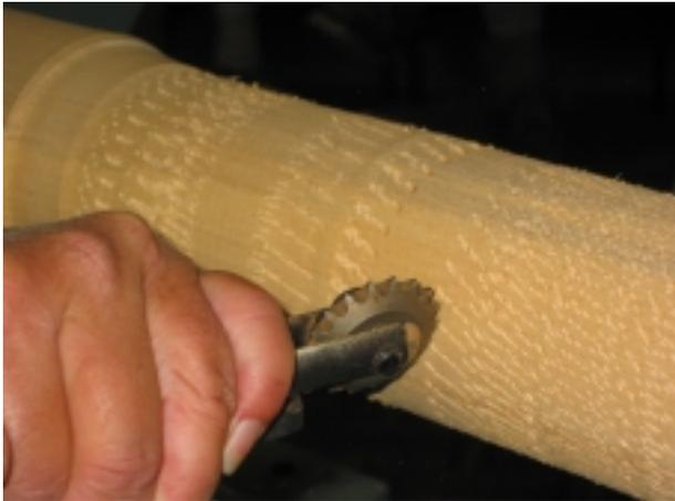
Next she added liming wax while noting the shoe polish and other coloured additives that fill the pattern made by the texturing tool are also good.
