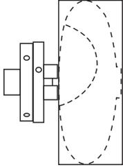
Create a spigot on the upper side of the planned bowl. Do this between centres or by gluing on a waste block. The off-set bowl may be planned to allow the use of a screw chuck, but a faceplate will not work. Turn the underside like a normal bowl. Keep the foot nice and flat and a full 1/3 of the width of the bowl. Sand and finish this side.
