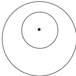
Take the wood off the lathe and work out exactly where the centre of the offset bowl is to be. Mark this point clearly.
