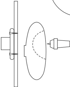
Mount a large faceplate of mdf on the lathe and glue the work piece to this. Put the center of the planned offset bowl to the point of the tailstock live centre. Then move the tailstock and bowl wood up to the mdf. If you are quick, you can make a puddle of hot melt glue on the mdf before bringing up the bowl wood. The foot of the bowl should be flat on the mdf, or you may try a little sloping of the work.
