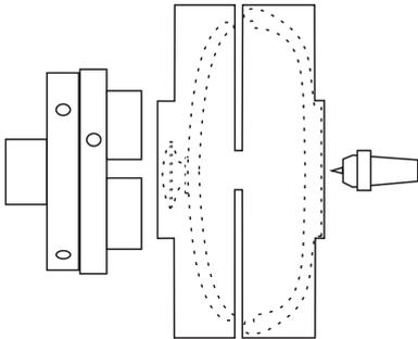
Mount the chosen wood between centres. Round it off and make a chuck bite spigot on both sides. Mount this in a chuck by the side planned to be the top of the box.
