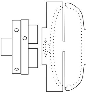
If the spigot on the underside of the box is to be retained as the foot then you may completely finish the part that is to be the underside of the box before parting it off.
