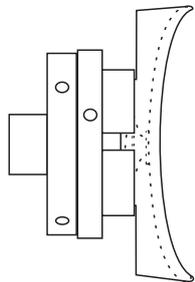
Cut the diameter of the top down to the exact size required to fit the bottom.
