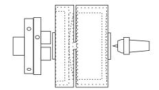
Mount the chosen wood between centres. Round it off and make a chuck bite spigot on both sides. Mount this in a chuck by the side planned to be the top of the box. The plan is to complete the outside of the bottom of the box later, so just part the two halves of the box. Set the bottom part of the box aside.
