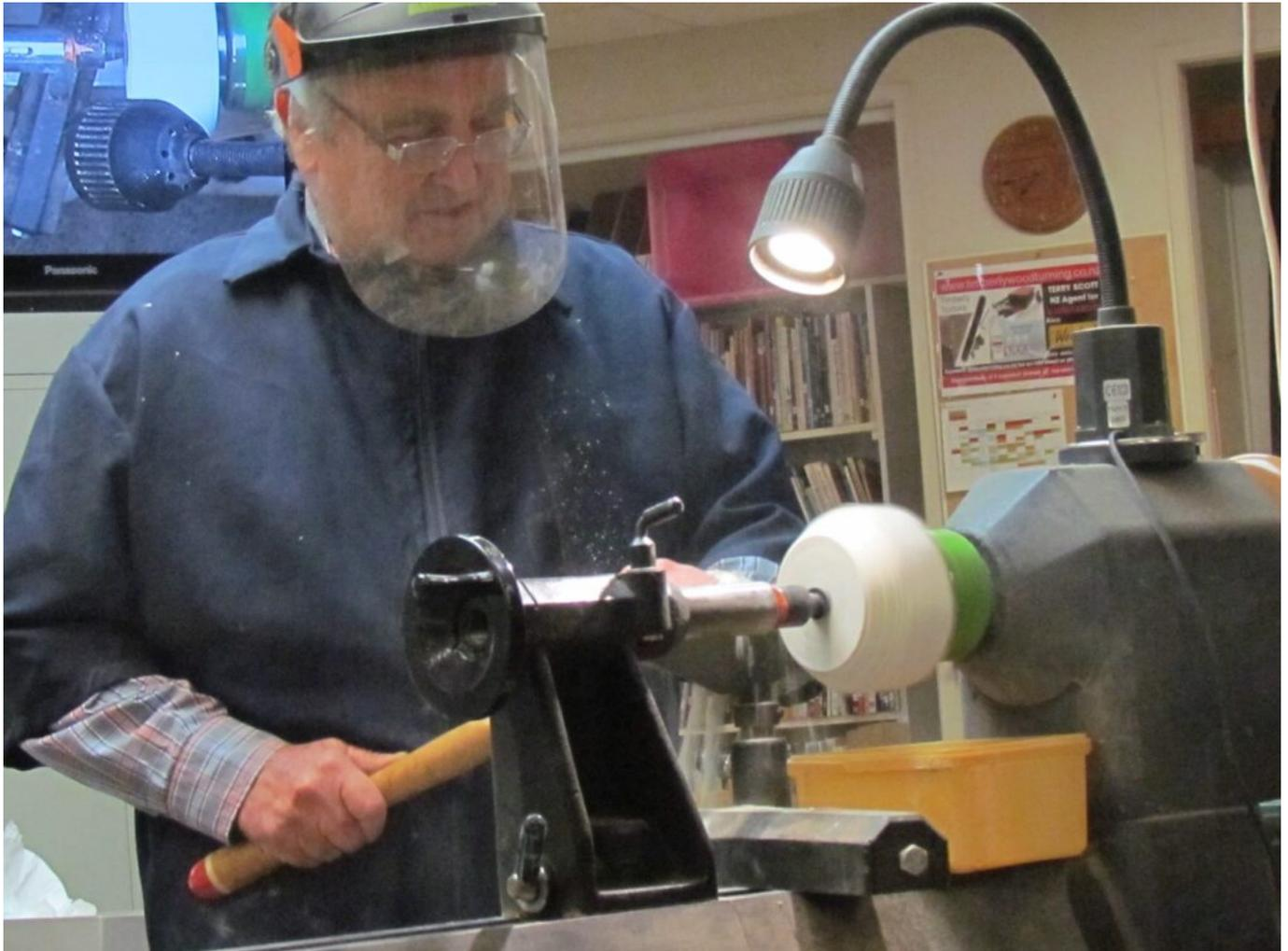
The stone was turned at a slow speed, and normal woodturning gouges were used. Containers were placed under the lathe to collect the dust, which would be used later for the lid.
