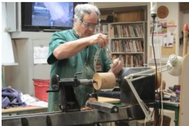
The cylinder was marked. In this case 124 mm. The length of the cylinder is now the same as a diameter and sitting between two centres. The new cylinder marked using the Soren Berger tool. The first cut was made straight between the two lines marked on each face - and using specialist tool.
