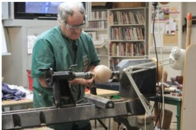
Then, second lines and marked using the third part of the specialist tool or caliper. The cuts then straight lined between the marks. The sphere is starting to emerge. These new lines are now the high spots on the proposed sphere.
