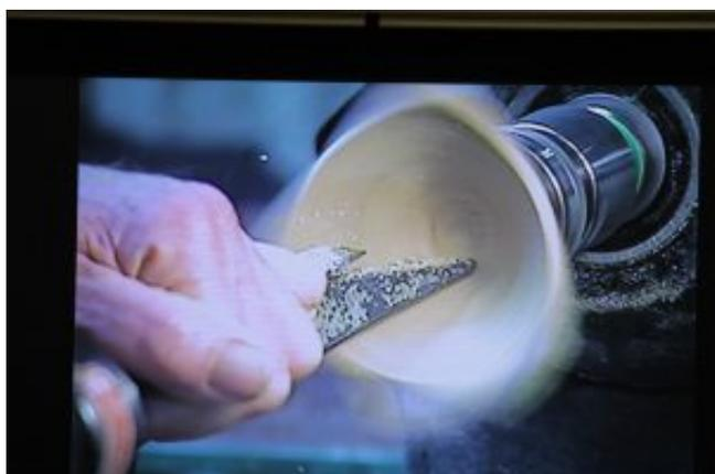
Colin pointed out the tearout that is inevitable in turning a cross-grained bowl, and suggested using sanding sealer during the final cuts, to minimise this. He then described finishing the outside and the foot with the bowl held between centres using cushioning at the headstock end to protect the inside surface.
