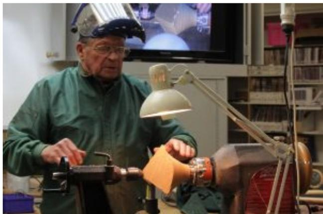
He then turned away the wood that was now at the tailstock side of the three points, creating three wings. When the spindle of waste between the points and the tailstock became thin enough, Colin knocked it off and then turned the inside of the bowl at higher speed (about 1400 rpm) using a cup tool, thinning the wings at the same time.
