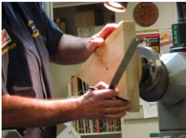
The back of the three sided bowl can be marked with the same markings as already described above. Go to the band saw and cut from apex to the marked centre on the three legs. There are many ways to sand up the three pieces but the sanding disc on the lathe with a supporting table on the lathe bed which was demonstrated worked real well. Sand each piece, round the corners and do the top and bottoms. In other words finish all the sanding at this point.
