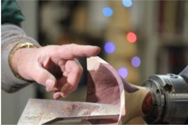
Final exterior smoothing is done with a curved scraper. When completed the piece is turned around with the narrow end of the vase at the headstock end so that hollowing can begin. First the spigot is cleaned off and then normal bowl hollowing and smoothing takes place. Watch fingers with those flying vase “wings”! As hollowing proceeds, care is needed to ensure the bowl thickness is evenly distributed to conform to the outer curve. Use the callipers.
