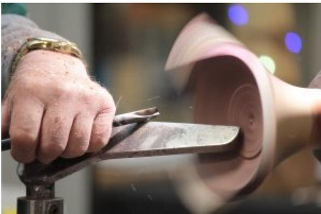
Once the spigot has been made the block is removed and remounted in the chuck (using the aforementioned mark). Now the tailstock end of the block is shaped to a flat surface so that the live centre can be brought up to the block with the jam chucks now discarded. Now another spigot is formed at that end (45 mm for a 50 mm chuck). When completed the block can later be held each end by chucks.
