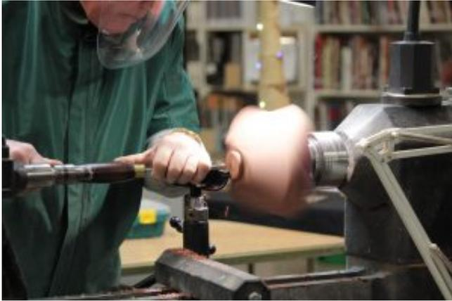
First step was to turn a spigot on the headstock end of the block, held by jam chucks between the main chuck and live centre, and using a bowl gouge for most of the shaping. Make sure the piece is marked so that it can be remounted in exactly the same position. Using a high r.p.m. Cam made the first cuts into the top third (nearest headstock) of the block to fashion the spigot. Keep moving the tool rest so that it is always as close as possible to the work to prevent “chatter”.
