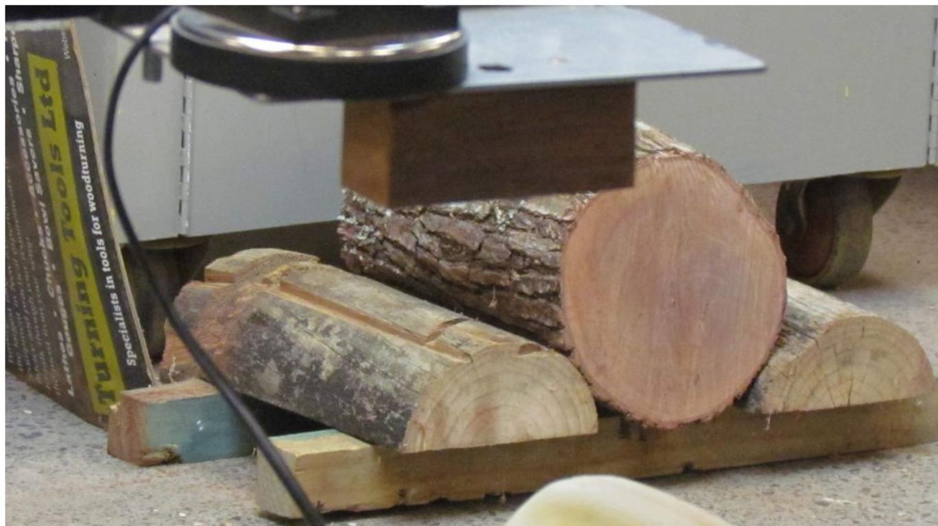
The chainsaw settings: Teeth at 30 degrees for cross cut, and along grain cutting.
