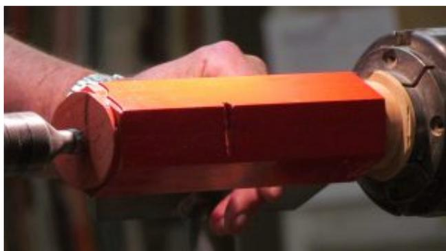
Back to the top i.e. the sharp end that that has imitation graphite in it. The lip is mark with Vernier callipers and cut down with a standard skew. It is hoped that you have remembered to leave sufficient thickness to accommodate the flat faces and that they join into a new top.
