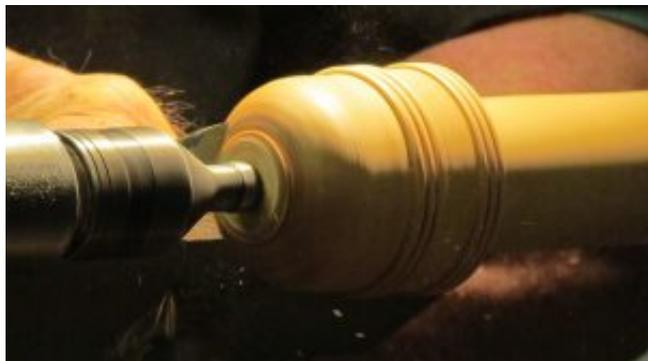
The finishing touch: The bead lines highlight the end of the pencil in the piece that holds your eraser. Texturing highlights these beads provides a differentiation to the pencil part and hopefully shows up in its glory, with some clean edges. This part of the process is achieved by putting the top of the box/pencil case onto a cylinder mandrel. Holding the box top on with the stem centres will assist safety and avoid any mishaps.
