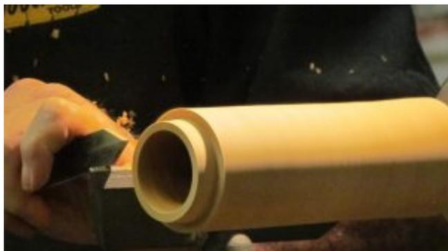
The next process is started with hollowing by way of Forstner bit or bits if you are precise. A piece of measured tape on Forstner bit provides a depth check. The second Forstner bit opens the hole further. The second part of the hole is continued with an extension on the Jacobs chuck.
