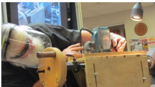
The pencil faces: Dick brought out his cleverly fashioned jig. A boxlike structure that is attached to the frame of the lathe. After some adjustment, fiddling, shifting around, the Router was used to clean off the six faces of the pencil. Some measuring and judging is required. The box is relatively simple and is technically only a guide for the router. It is simply one of the ways in producing the six sides of the pencil - all hopefully matched even and appropriate looking.
