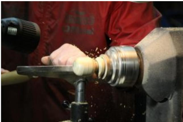
Despite the decent sphere which was produced Johns ended up adopting the quote “What you lack in skill you make up with a bit of brute force and sandpaper” and he proceeded to grind the ‘sphere’ down to a sphere using a cut steel pipe, it was then finished off with ondina oil and sand paper.
