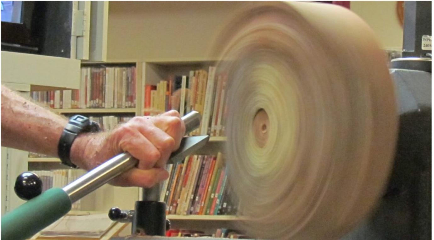
John went on to demonstrate how one would mount and turn a conventional wet half log. He covered briefly how to cut bowl blanks to get different grain patterns within the bowl, butterfly or oval rings etc. John then used a faceplate to attach his large Rewarewa log to the lathe. He prefers to use passivated Tek screws over galvanised, as they are less likely to shear and they come in a great size range.
