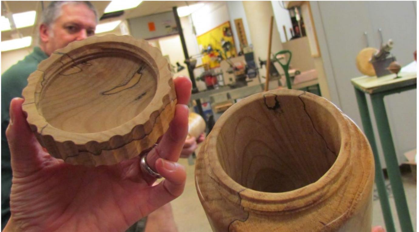
On completion of the threading and the box, Dick with his router made a fluted edge around the edge of the lid to hopefully show people using the box, it was a screw lid and not a pop lid.
