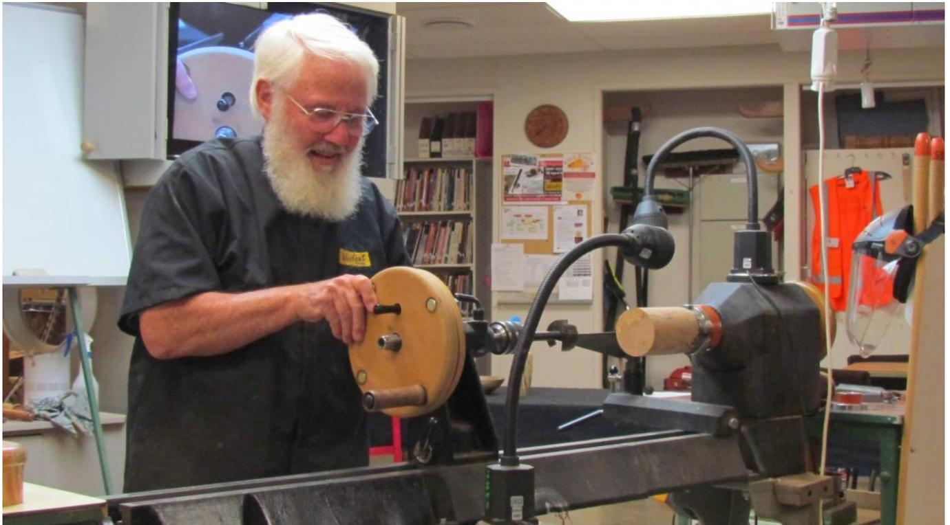
Dick used Taraire wood and turned the basic shape of the outside of his box. Then used a forstner bit to take the box centre out. A large wooden jig was placed over the tailstock handle with its own extra large handle, to help keep a more consistent turn of 230r while drilling. A consistent turn helps for a better drilling result. He used Boelue lube on the bit to reduce the squeal.
