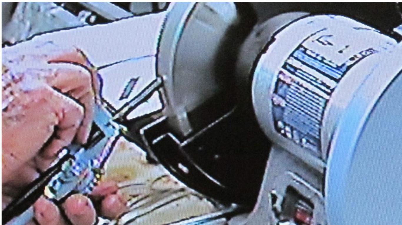
The usual form of abrasive wheel sharpening is via a double-ended grinder having wheels of 150mm (6") or 200mm (8") diameter, the larger size being preferable but more expensive. More specialised machines are available including several brands with larger 250mm (10") wheels running in a water bath and slower speed grinders intended to reduce the generation of heat.
