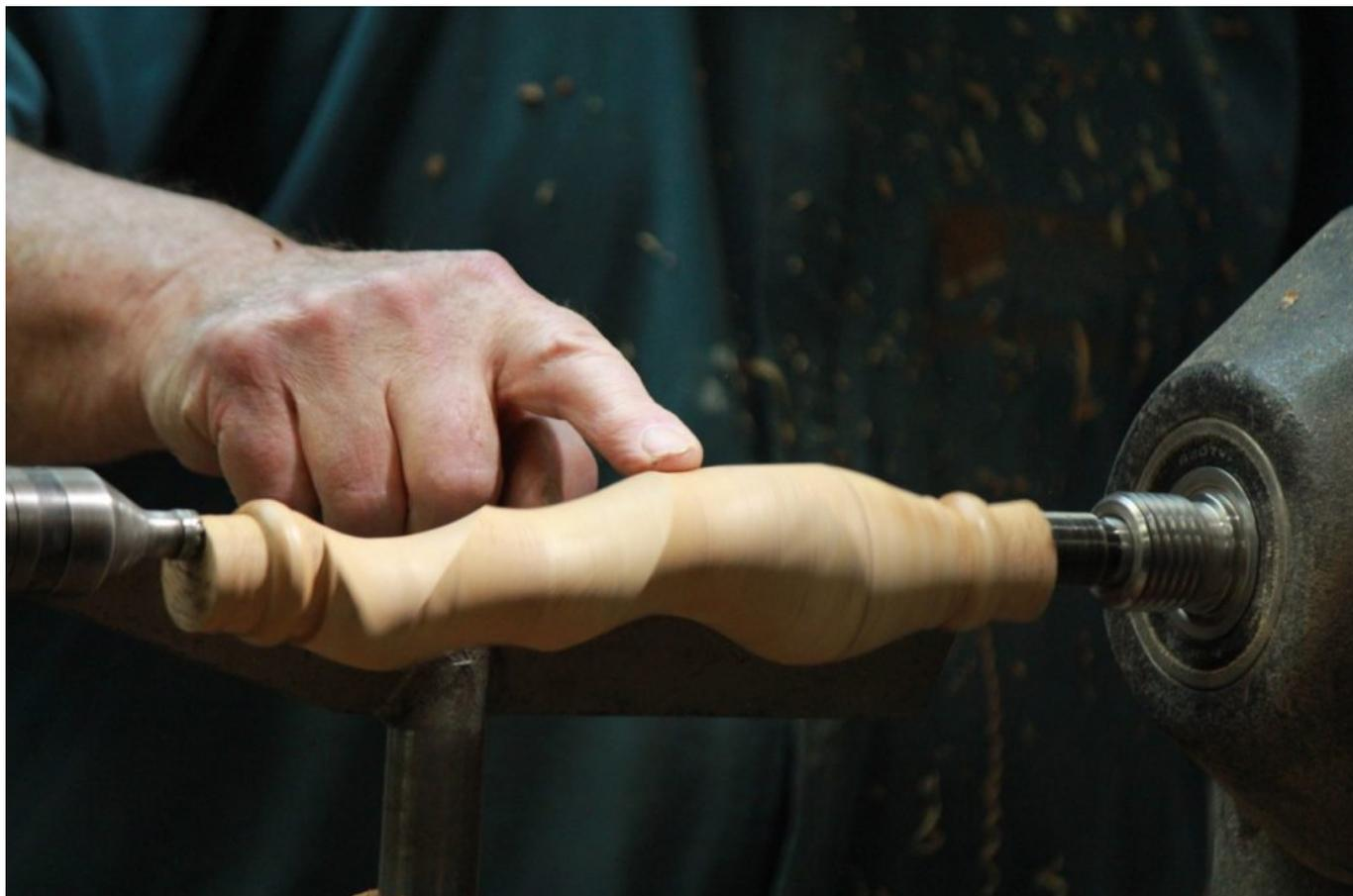
With the next spindle blank, Dick marked the centres and then measured 10mm out from centre on the diagonals and made four equal marks. He numbered them 1-4 clockwise. He repeated this step on the other end of the spindle, but off set the numbers by  $\frac{1}{4}$ . He then mounted this between Stebs and rounded it leaving a fair amount of width to the spindle. He took about 20mm at each end down to a 40mm width and made a bead at the end of each section.
