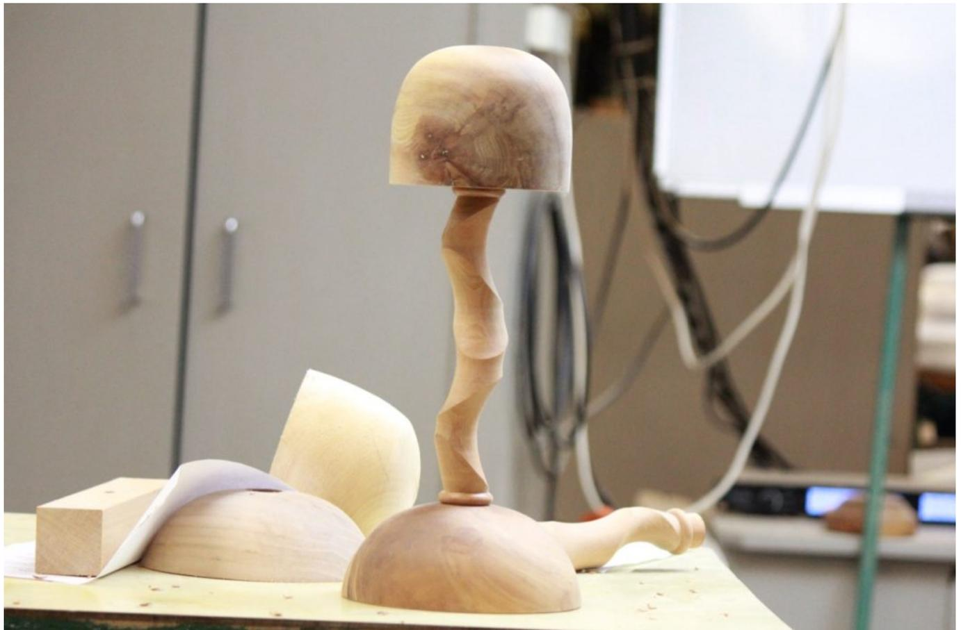
Upon finished the last section he stopped the lathe and inspected the result to see if there were any remaining flat spots or areas that needed tidying up. Once satisfied, the spindle was complete. It really was an incredible 'drunken twist' formation that really made the viewer question how it was made. Great demo thank you Dick, it was my first time seeing off centre turning and it has given me a lot of inspiration to give it a go.
