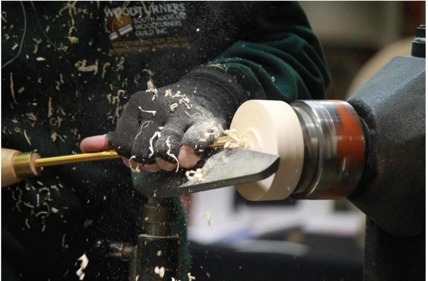
Once the bottom has been turned to desired shape, David separates it from the lid (top) and removes it from the lathe. He then remounts the lid in the chuck and cleans off the face. He carefully marks the diameter of the bottom on this face and proceeds to hollow the lid. Aiming for a snug fit, slightly on the loose side so it won't jam. To achieve this it is essential to work slowly and measure constantly.
