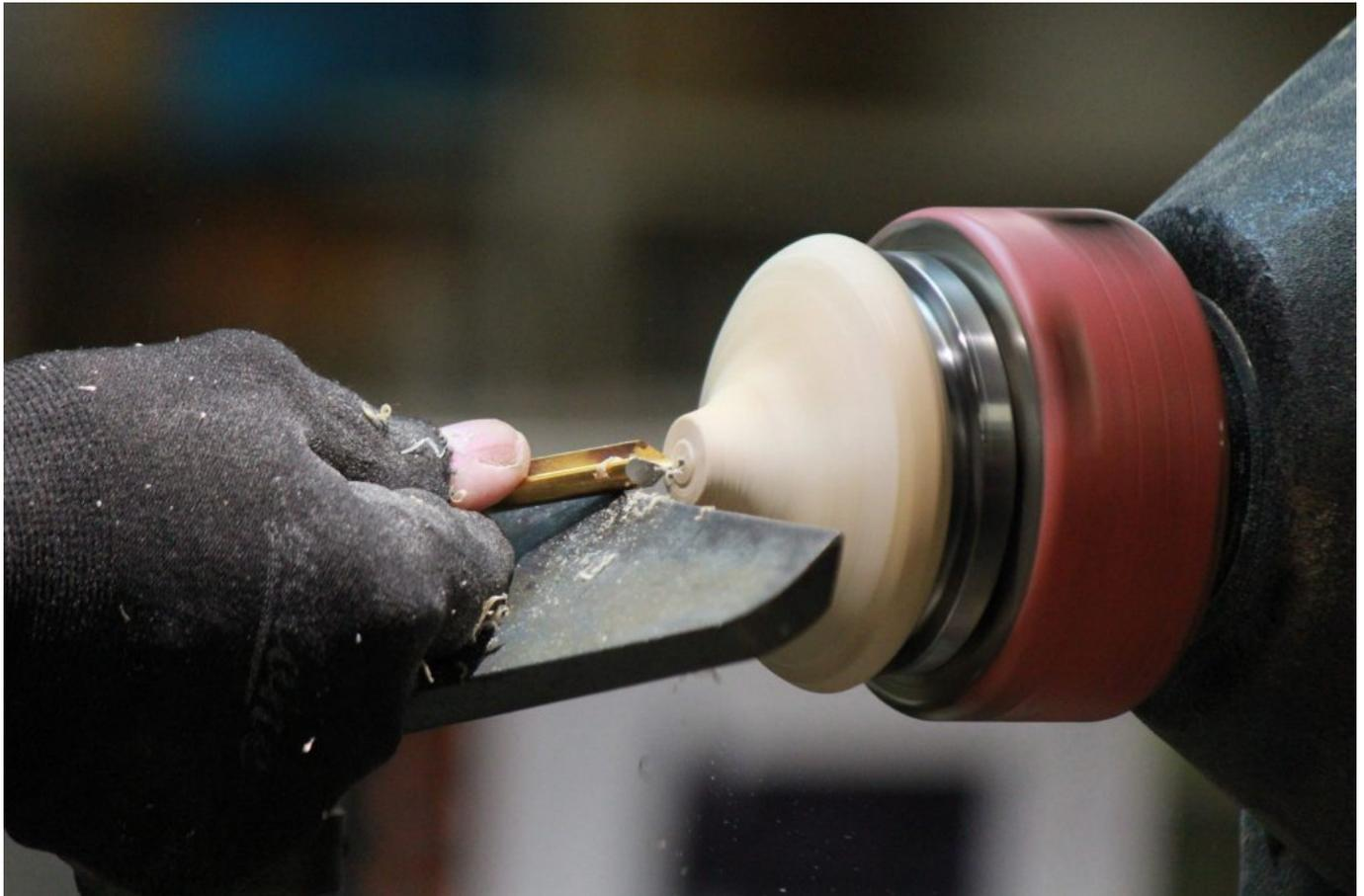
Next step is to re-mount the lid on a smaller chuck gripping the inside of the lid and using tape or sheet rubber to avoid marking the rim. A jam chuck is another alternative holding system. Now the exterior finishing can be completed. This includes drilling a suitable sized hole (6 mm) for the addition of an ebony knob or finial which will be glued into the hole.
