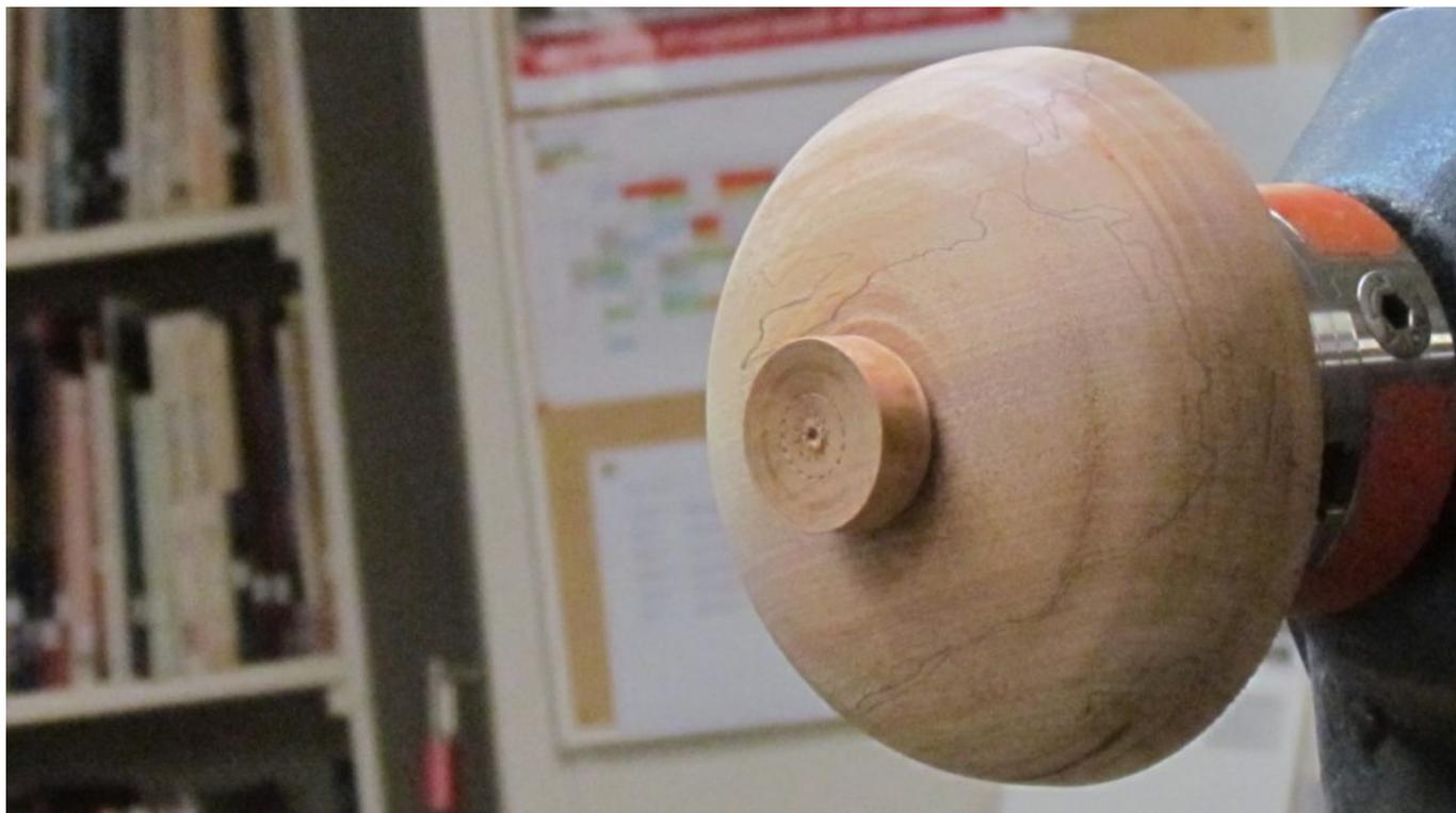
Then take the base spigot off he used a wooden plug that fit into the 25mm hole and then held the plug in the chuck and turned it off. Colin noted here that its best to make a slight concave so contact points of the base are the perimeter only. This will prevent wobbling and give stability when there's a heavy wet wig on top.
