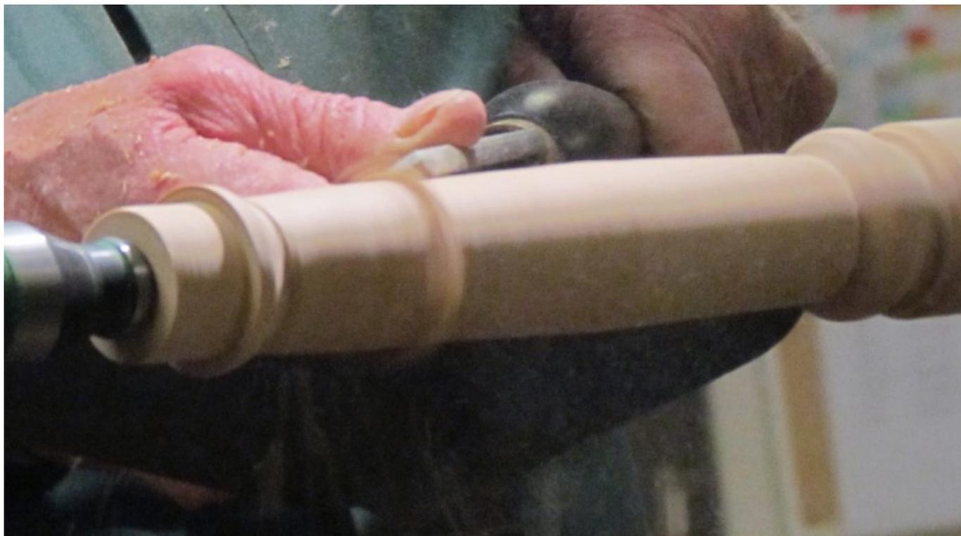
Colin demonstrated that this was also an excellent time to practice using the skew chisel when shaping the shaft.
