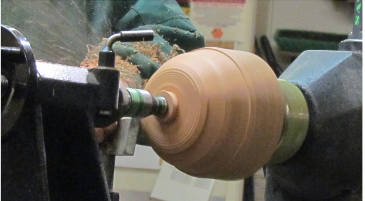
With the base finished, Colin moved on to the head. This piece was a 160 x 110mm square, noting to use a light weight wood for the top. Colin used a steb centre to hold the piece while shaping. He mentioned here that it is important to make sure the edges of the top are either parallel, or slightly curved under so as not to have a protruding edge that would damage a wig.
