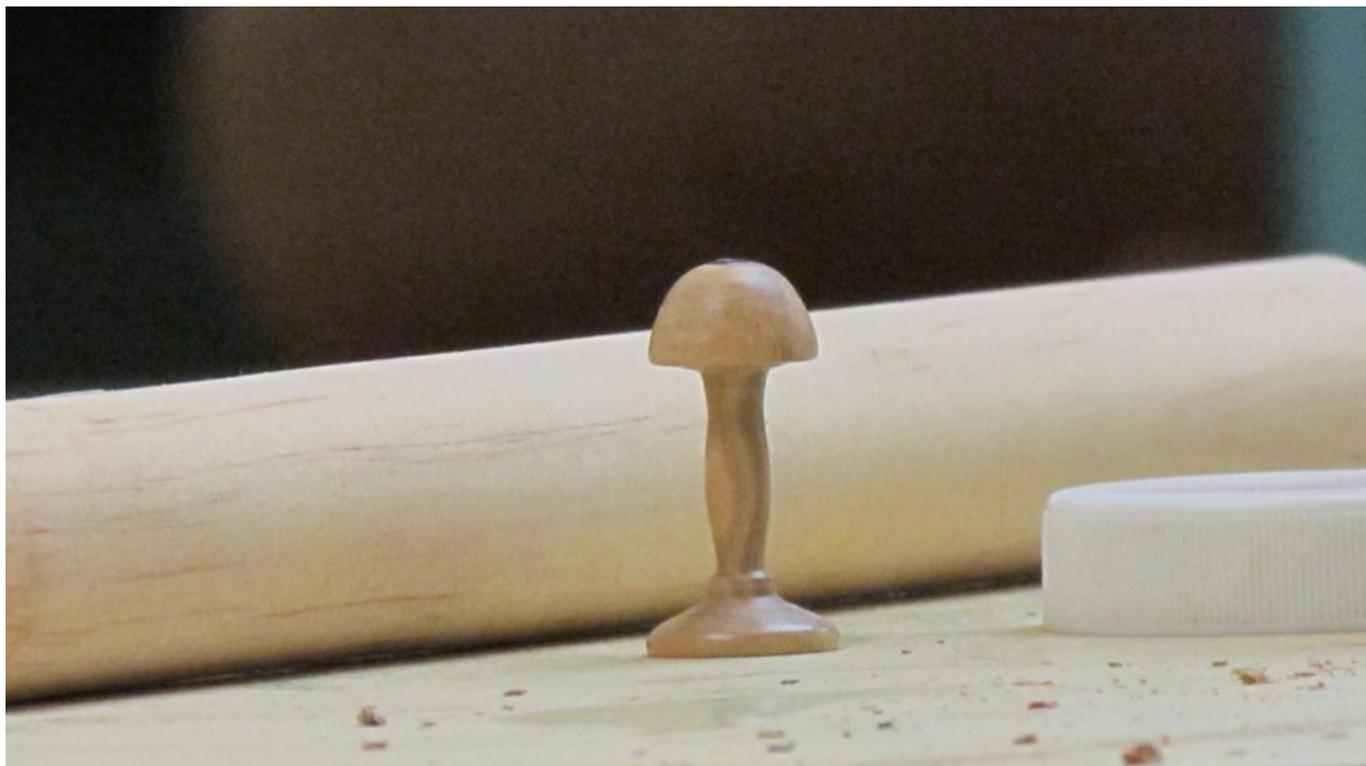
Colin then started out by making the base section first, using a square 160 X 50mm block of spalted Taire timber. He'd already drilled a 25mm hole, in which the stand will fit, and made a spigot on the other side. Turning at a speed of 800 he proceeded to round it off and then shape the base, noting that it is personal preference what shape/decoration you make.
