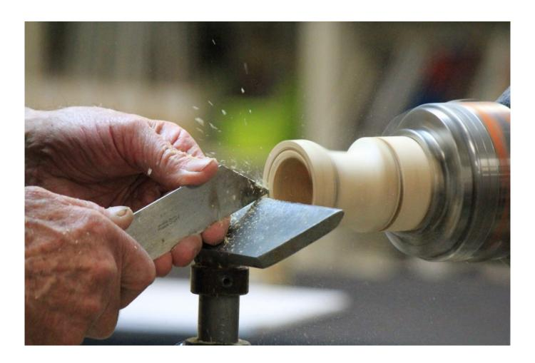
[HANDY TIP No. 3: When turning shapes, rebates, etc., to fit other shapes and rebates, keep checking for a good fit as you go along. Very easy to take off too much and lose a tight fit.]
