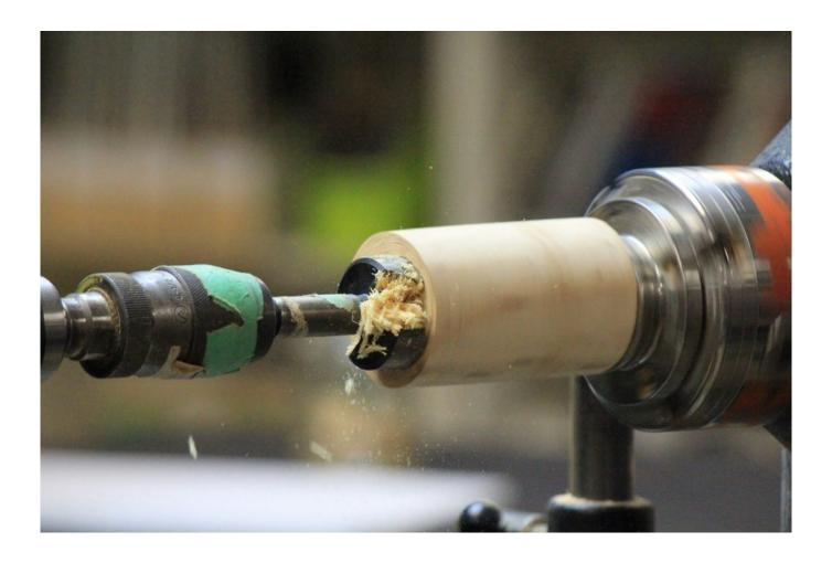
[HANDY TIP No. 1: Colin uses boelube on the drill to keep it moving and avoid burning. Always drill slowly with Forstner bits and frequently extract from the hole to clear shavings.]
