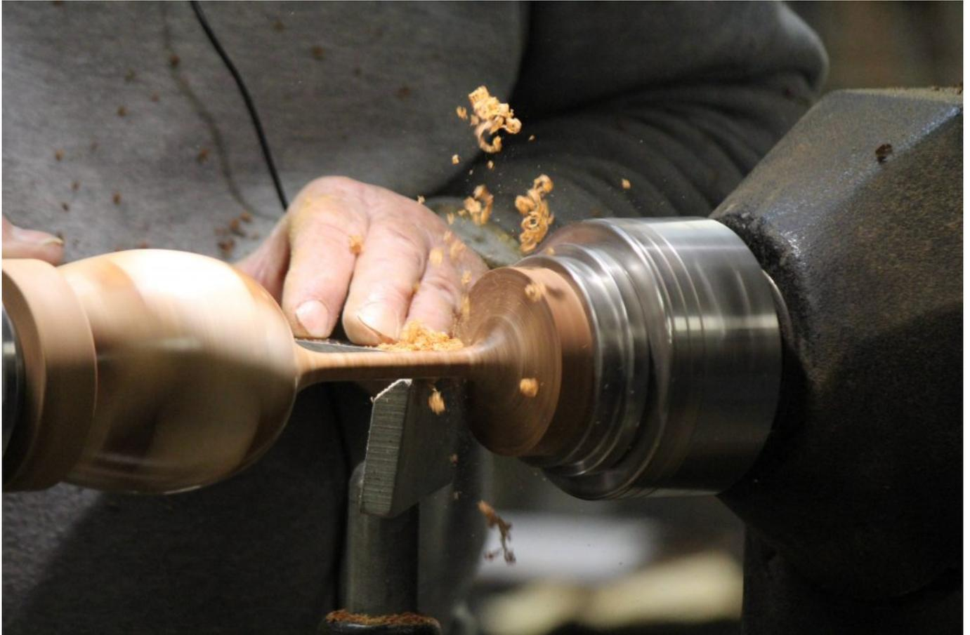
As the stem became slimmer, Cam's work became increasingly careful, taking off small bites of timber (more like dust than shavings) to avoid a disastrous jam and a ruined masterpiece. Eventually he got it down to his planned 5 mm diameter and finished with sandpaper.
