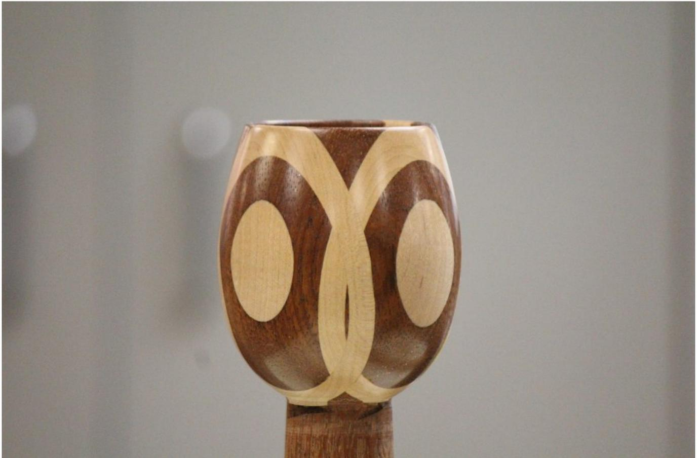
As with all projects it is important, Cam teaches us, to start with a plan drawn to scale. The first task is to cut four slots in the bowl end of the goblet block using a drop saw. To prevent the cut intruding into the stem of the goblet Cam has devised a jig which keeps the block sufficiently far from the saw backstop to prevent this happening. All meticulously measured of course. The wedge shaped cuts are to take the maple lamination inserts.
