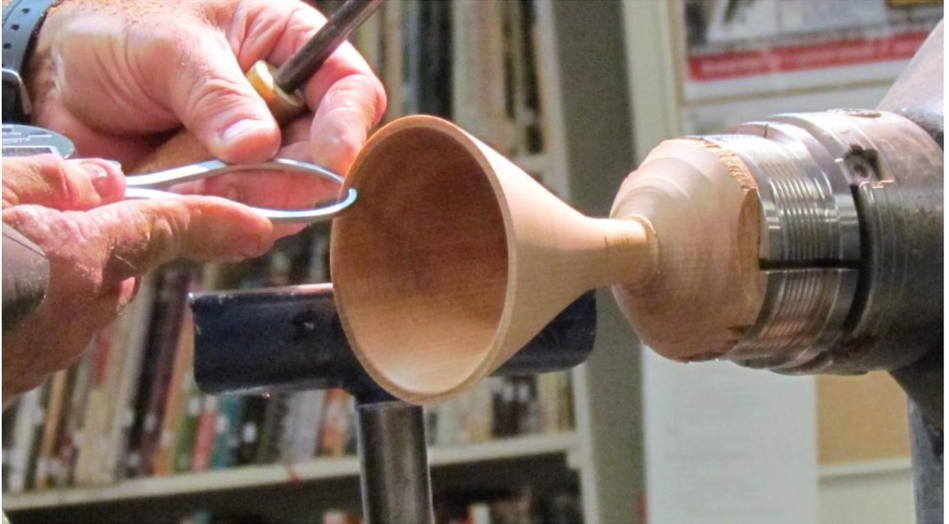
Now he drills the 8mm hole the rest of the way through the tube end of the funnel, taking care not to have the drill chuck scrape against the finished inside walls. To do this he had to progressively pull the drill out of the chuck until it was almost wobbling in space. A drill extender might be the answer.
