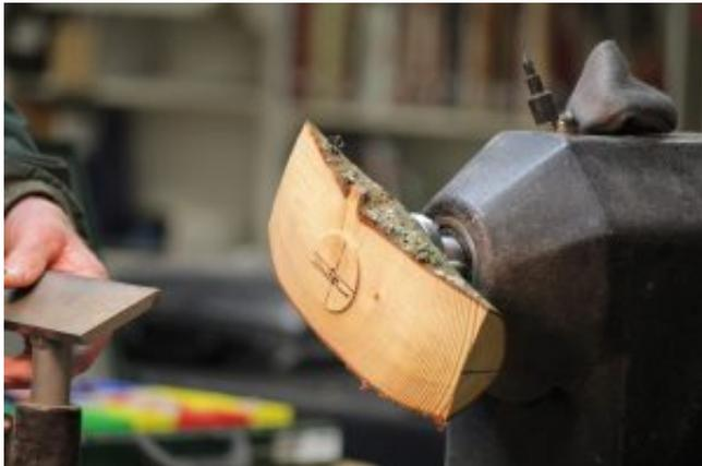
A tip for sanding: Chris uses chalk gently rubbed across the face of the surface being worked to highlight and identify scratches, marks cuts and hollows. Chris used a standard soft builders chalk stick rubbed across the surface and using the marks to decide on the type and placement of the next cut. This process was used for final sanding with Chris providing illustration of what marks show through at the movement through the sanding paper grades.
