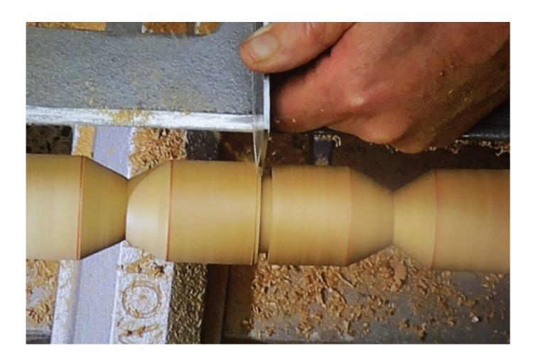
The cut was tidied up with a spindle gouge before being drilled out with a forstner bit.
