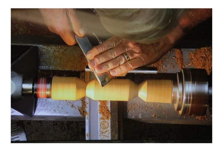
Once the cracker fits together firmly and snugly, the tail stock is brought up to support the entire cracker. Here you can tidy up the outside, so it is flush. It can now be sanded and textured however you prefer.
