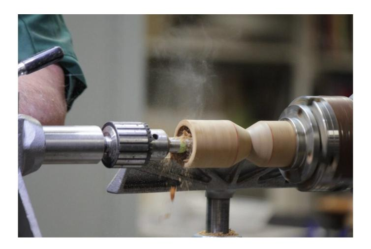
The outside ends of the cracker, and one of the insides were drilled out with a 38mm forstner bit. Drilled to a depth of 40mm.
