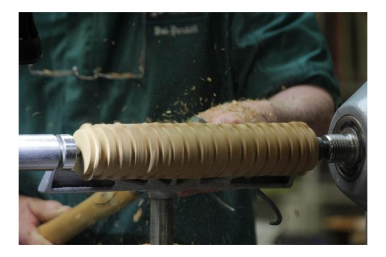
Spigots of 48mm wide by 8mm deep, were made on both ends.
