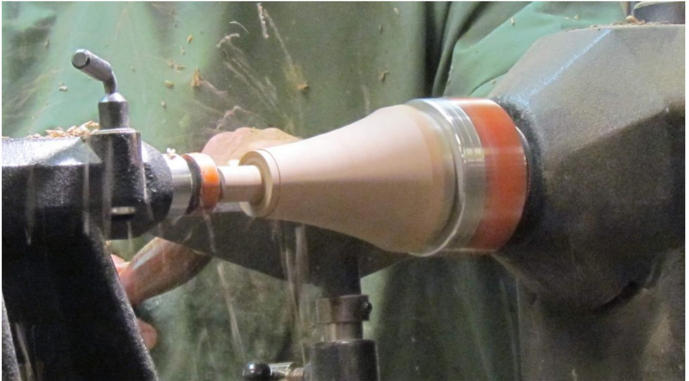
Once the base had been shaped, the next task was to turn the first platter to round. Bob fitted the base to the platter using the spigot and using the tail stock, pressed the platter against a large disc mounted on a faceplate. With the lathe running at a slower speed, this was a quick and effective method of holding the work for finishing.
