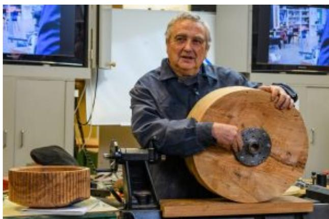
Once your monster slab(attached to a faceplate) is on the lathe, work is needed to shape the outside of the bowl before starting the lathe. Warwick used a Bosch electric saw which he won in a raffle to cut off the rough corners, followed by an electric planer, also won in a raffle, and finally a King Arthur sander.
