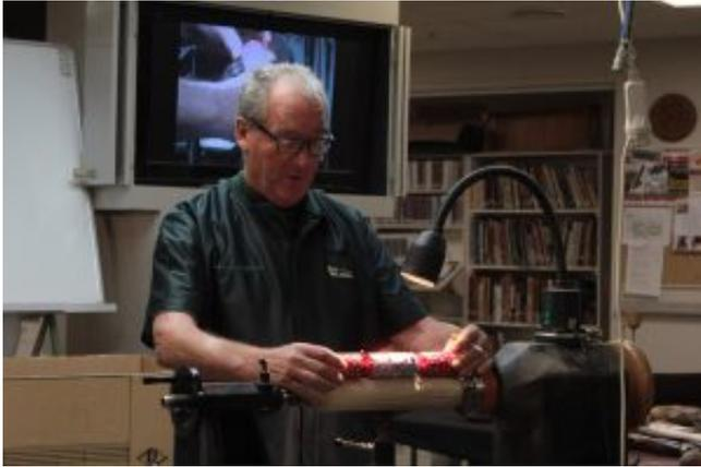
A turned cylinder with two chuck bites was marked into three pieces, i.e. two ends and the middle. Grooves cut to identify the ends and then the centre piece was parted in the middle. The centre and ends were then drilled out and the centre fitted back together as you would when making a lidded box. A hole was drilled through the narrow part of the ends so that the tail of the exploder could be passed through and glued into place when the cracker is assembled.
