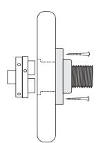
Screw the steel handwheel onto the material. You can now remove it from the chuck. Sand the edges of the drilled holes. Give the whole project a good coat of hard-wearing lacquer or varnish.
