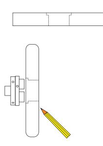
Mark the centre of your material. Drill a 54 mm diameter hole 5 mm into the material. Then drill a 45 mm hole completely through the material - this allows a knockout bar to be used. You may have to change these dimensions to suit your steel handwheel or if you are planning to use a vacuum chuck.
