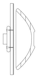
Take the bowl off the chuck, turn it over and remount it on a vacuum chuck, Cole jaws or other method. Cut, sand and finish the foot of the bowl.
