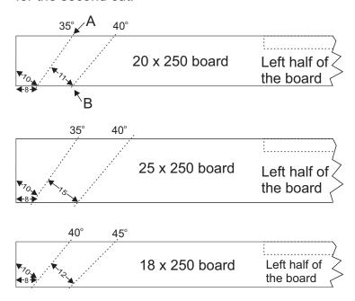
The measurements shown below are for a board 250 mm in diameter and 20 mm thick to show what parting tool you need to use - shifting the cut line is not an option. Each parting cut is to the right of the marked line. The angles are a clockwise rotation from vertical.
