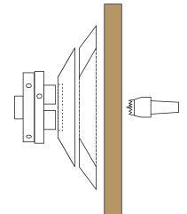
You now have the inner, smallest part of the bowl still on the chuck and three rings of wood. Take the smallest of the three cut rings and glue it, with perfect alignment, to the small part on the chuck. Bring up a board and the tailstock to press it into place until the glue is set enough to add each of the next rings. When the glue is set you can shape the bowl. Cut, sand and finish all the inside and a much as possible of the outside.
