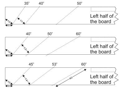
The first cut allows for a 4 segment bowl with a thickness of 10 mm but that can be continued only if a 1 mm parting tool is used for the first cut.
